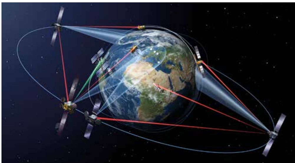
Figure 117: Schematic of the European Data Relay System (EDRS) 219
